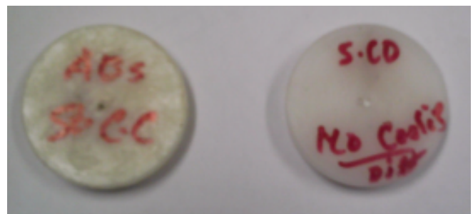
Fig-9 Sample test part produced for experimental verification Left: ABS right: PP plastic.
