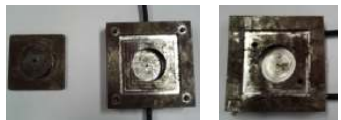
Fig-5 (a) Mild steel Core (left) and cavity with SSSCCC (b) CSCC of mild steel.
