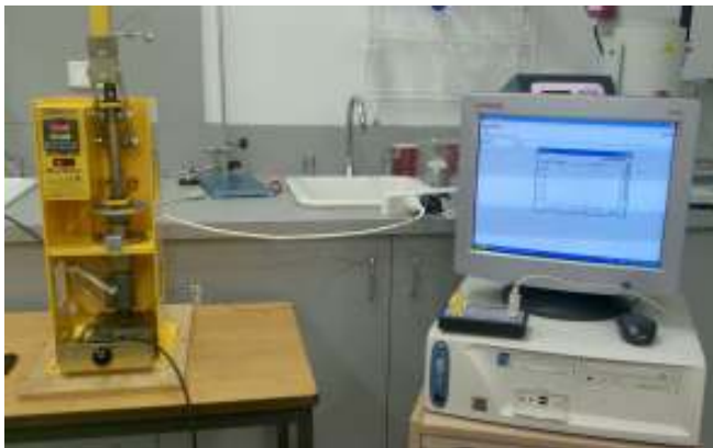
Fig-6 Experimental setup for test injection moulding, left: mini moulder, right: temperature output in PC.
