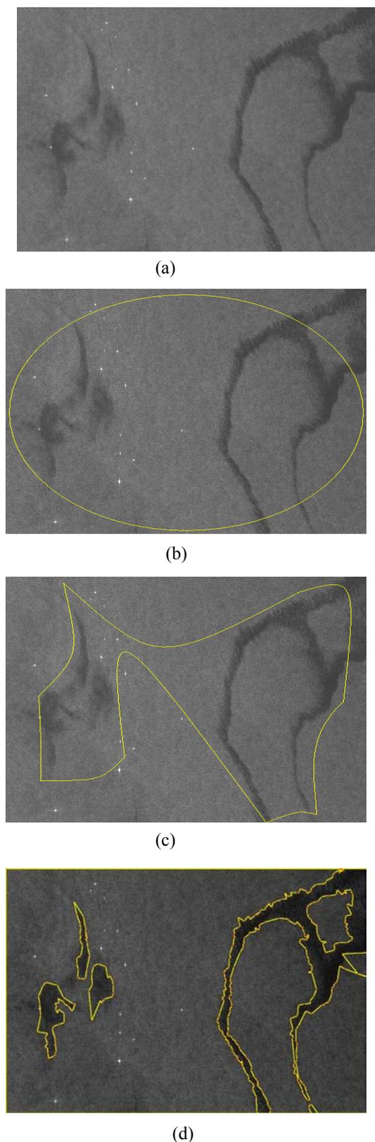
Figure 5: image segmentation (a) original image, (b) initial curve, (c) intermediate curve, (d) final segmentation
