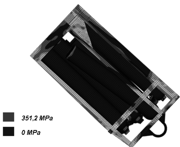
Figure 13: results in terms of Von Misses stress in the rotational falling load case.
