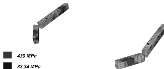
Figure 16: results in term of Von Misses stress in the rotational falling load case for the rectangular section where the bolts are connected
