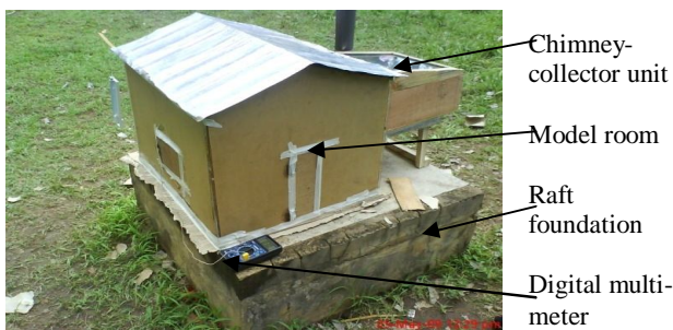
Fig. 2 Chimney-collector attached to the room
