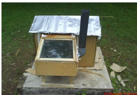
Fig. 3 Solar chimney attached with the building
