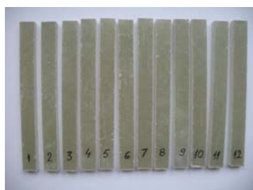
Fig. 7 Specimens prepared for bending tests
