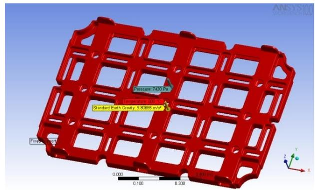
Figure 15: Loading and Boundary conditions on modified tray
