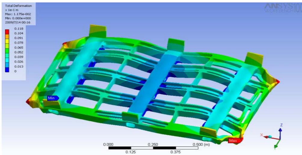
Figure 12: Deformation plot of existing tray(magnified X1000)
