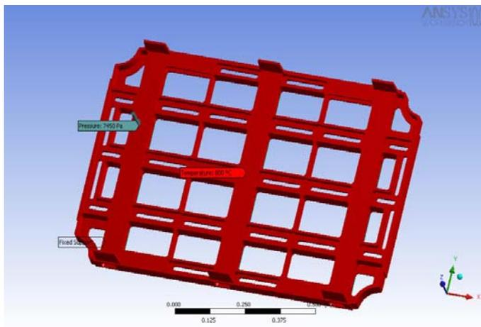
Figure 8: Loading and Boundary Conditions on existing tray
