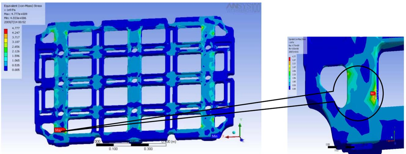
Figure 16: Stress plot of modified tray(right side shows the magnified view)
