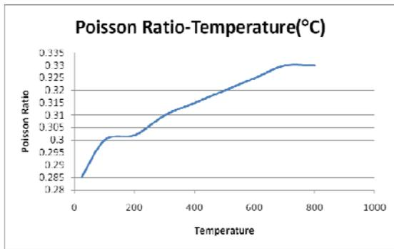
Figure 1: Poisson Ratio -Temperature Curve
