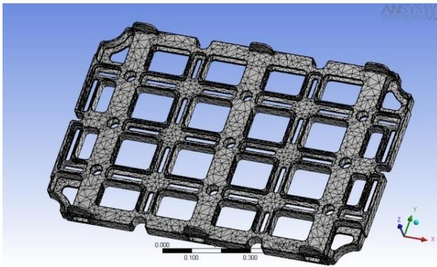
Figure 14: Meshed model of modified tray
