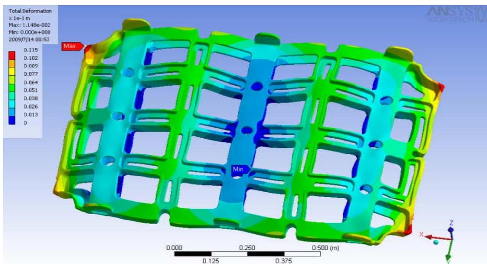
Figure 17 :Deformation plot of modified tray(magnified X1000)
