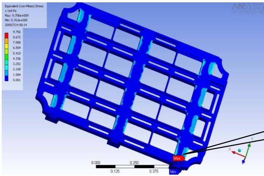
Figure 10: Stress plot of existing tray(right side shows the magnified view)
