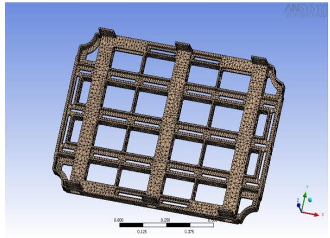
Figure 7: Meshed Model of existing tray
