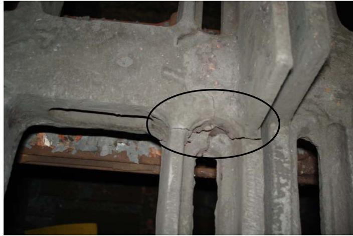
Figure 11: Photograph showing crack formation in high stress regions in existing tray
