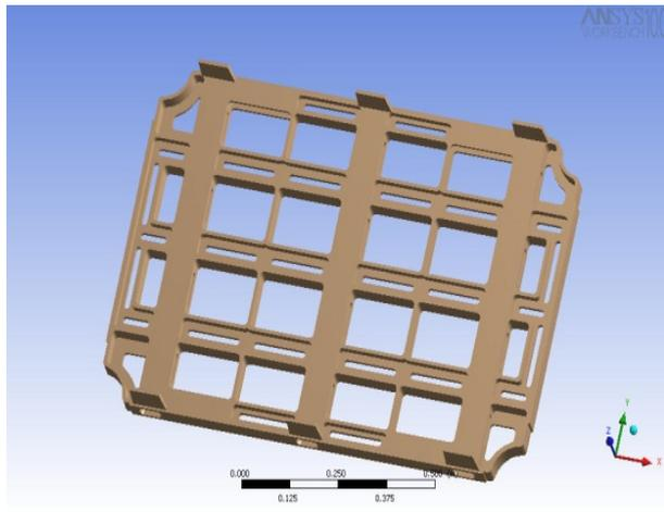
Figure 6: 3D model of existing tray
