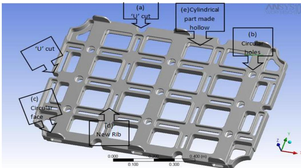
Figure 13: 3D Model of Modified Tray
