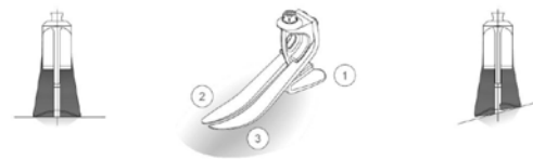
Fig. 2 Elite Foot prosthesis: 1, 2, 3 – components which are fabricated from composite materials like carbon fibber [12]
