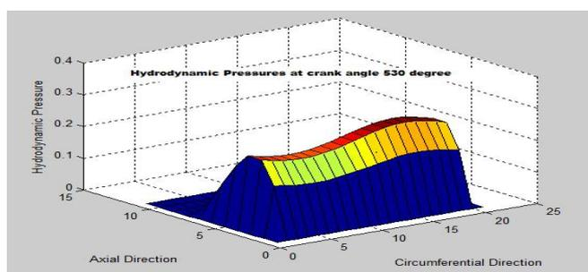
Fig: 9 Hydrodynamic Pressure Field at 530° Crank Angle
