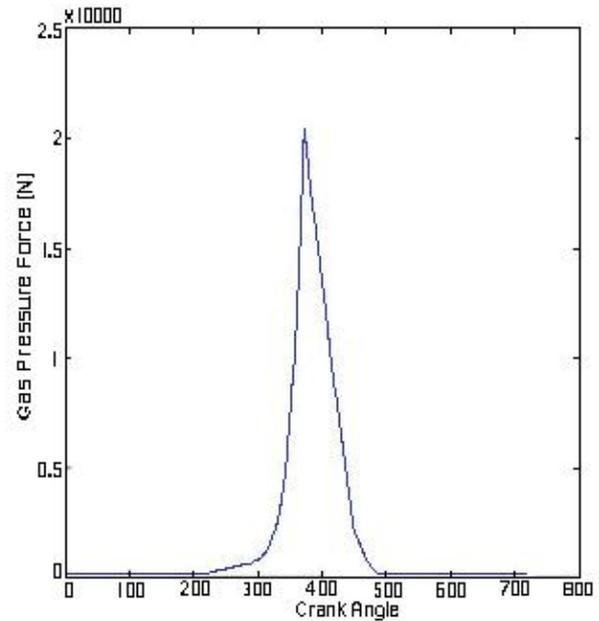
Figure:1 Gas Pressure Force Vs Crank Angle [11]
