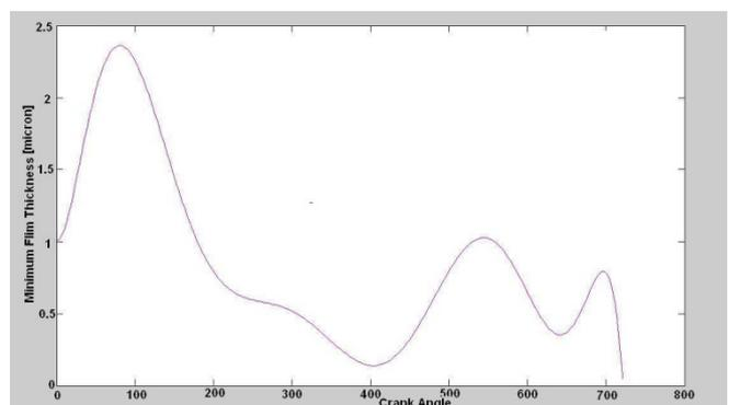
Fig:3 Minimum Film Thickness (Microns) Vs Crank Angle
