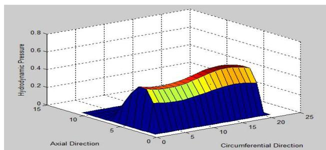
Fig:6 Hydrodynamic Pressure Field at 200° Crank Angle
