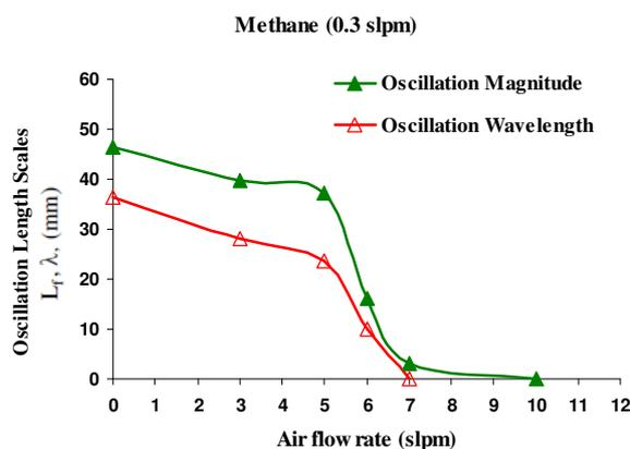
**Fig. 6:** Flame oscillating magnitude ( $L_f$ ) and wavelength ( $\lambda$ ) generally decrease towards zero by increase in co-flow air.
