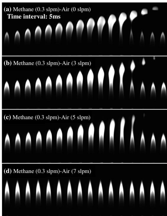
**Fig. 3:** Full cyclic sequences of high speed images of methane (0.3 slpm)-air diffusion flames at increasing co-flow air rates; (a) 0 slpm, (b) 3 slpm (c) 5 slpm and, (d) 7 slpm. The time interval between two consecutive images is 5 ms.
