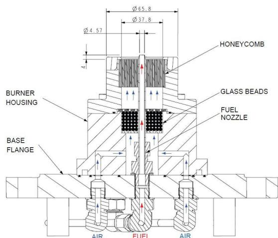
Fig. 1: Cross-section of the co-flow diffusion flame burner.
