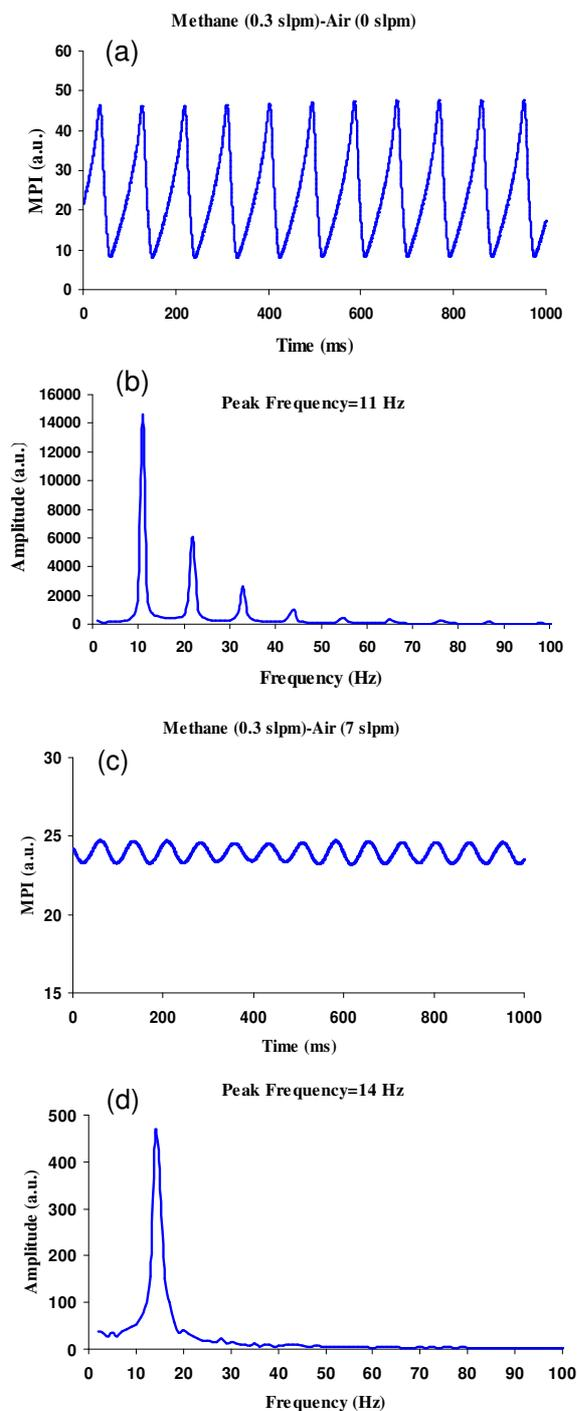
**Fig. 7:** Mean Pixel Intensity (MPI) and the corresponding flicker frequencies of methane (0.3 slpm) diffusion flame without co-flow air (a and b respectively) and at 7 slpm of air flow rate (c and d respectively).
