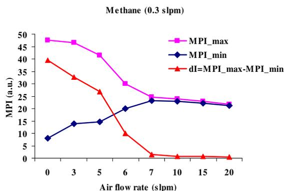
**Fig 8:** Maximum and minimum values of mean pixel intensity (MPI) from the flame high speed images in a whole cycle of the flame oscillation (methane (0.3 slpm) at different air flow rates). The subtraction of these two parameters (dI) decreases towards zero at the suppression air flow rate (10 slpm) and onwards.
