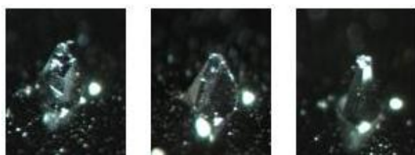
Figures 10 - 11 - 12: Stereomicroscopy images of failed microneedles according to M1, M2, and M3 failure modalities.
