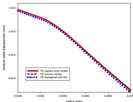
**Fig. 14 Comparison of residual radial displacements for mono fiber square and circular and hexagonal models**
