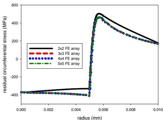
**Fig. 16** Convergence of residual circumferential stresses for different square arrays
