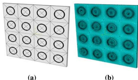
Fig. 6 a) multi fiber 4x4 square array RVE model. b) finite element mesh
