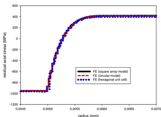
**Fig. 13 Comparison of residual axial stresses for mono fiber square and circular and hexagonal models**
