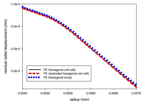
**Fig. 22** Convergence of residual radial displacements for different hexagonal models
