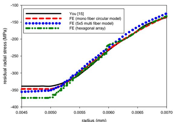
**Fig. 23 Comparison of residual radial stresses for different models**
