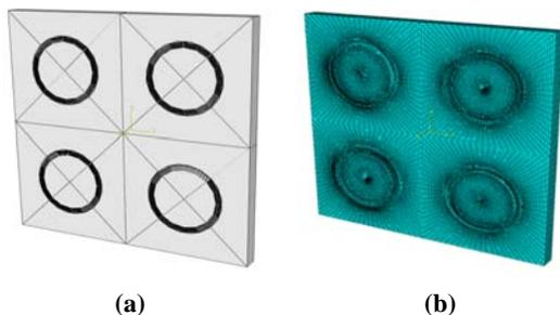
Fig. 4 a) multi fiber 2x2 square array RVE model. b) finite element mesh
