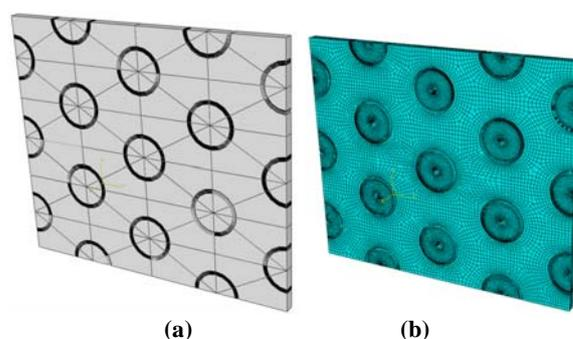
Fig. 10 a) hexagonal array. b) finite element mesh
