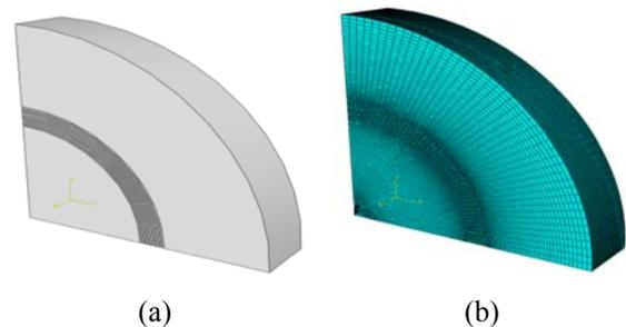
**Fig. 2 a) One fourth mono fiber circular RVE model. b) finite element mesh**
