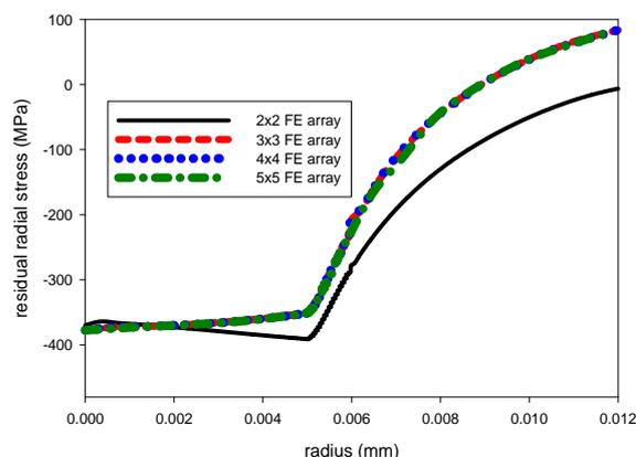
**Fig. 15 Convergence of residual radial stresses for different square arrays**
