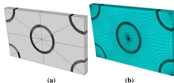
Fig. 9 a) extended hexagonal unit cell. b) finite element mesh
