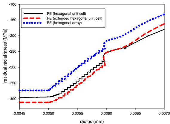
**Fig. 19** Convergence of residual radial stresses for different hexagonal models
