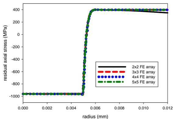
**Fig. 17** Convergence of residual axial stresses for different square arrays
