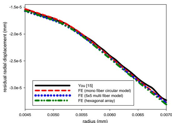
**Fig. 26 Comparison of residual radial displacements for different models**
