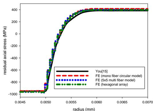
**Fig. 25 Comparison of residual axial stresses for different models**
