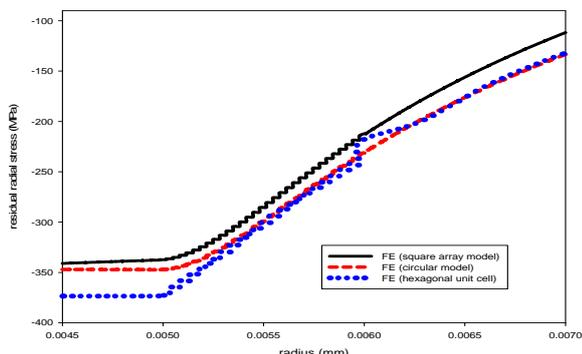
**Fig. 11 Comparison of residual radial stresses for mono fiber square and circular and hexagonal models**
