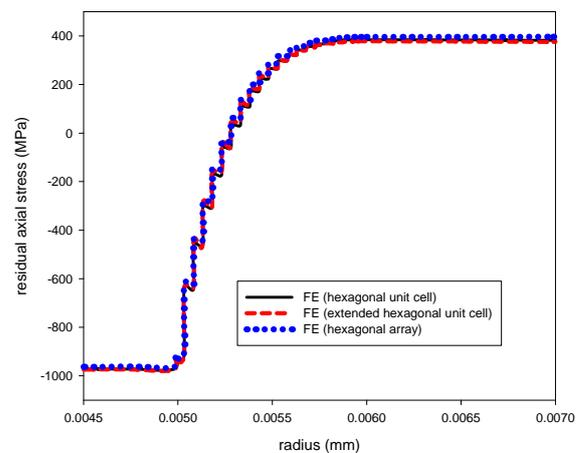
**Fig. 21** Convergence of residual axial stresses for different hexagonal models
