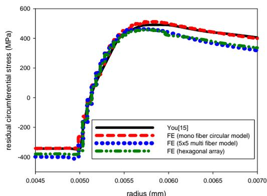
**Fig. 24 Comparison of residual circumferential stresses for different models**
