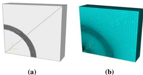
Fig. 3 a) One fourth mono fiber square RVE model. b) finite element mesh
