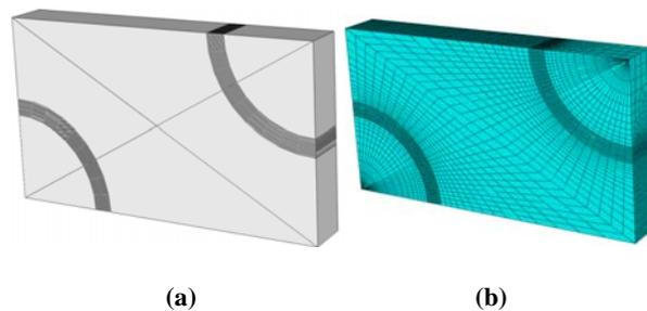
Fig. 8 a) hexagonal unit cell. b) finite element mesh
