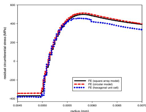
**Fig. 12 Comparison of residual circumferential stresses for mono fiber square and circular and hexagonal models**
