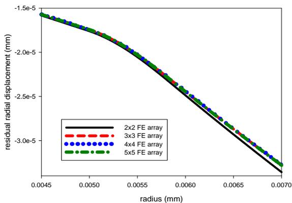
**Fig. 18** Convergence of residual radial displacements for different square arrays
