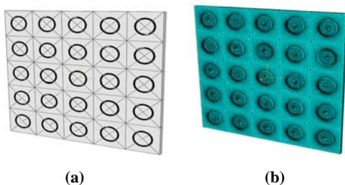
Fig. 7 a) multi fiber 5x5 square array RVE model. b) finite element mesh
