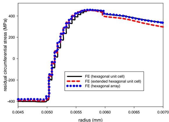
**Fig. 20** Convergence of residual circumferential stresses for different hexagonal models
