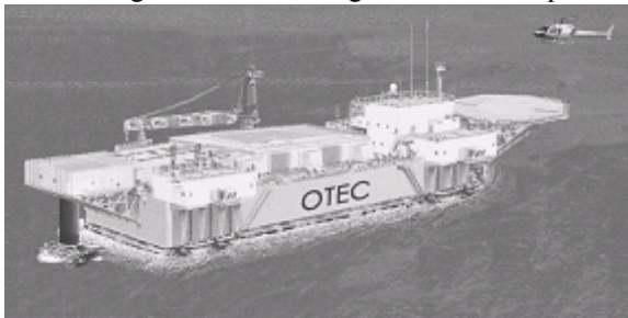
Fig. 2 Large Offshore OTEC Plant
