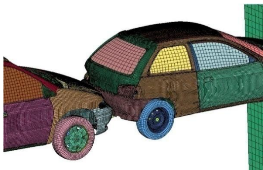
Fig. 3. The FEA results of the impact between two cars
