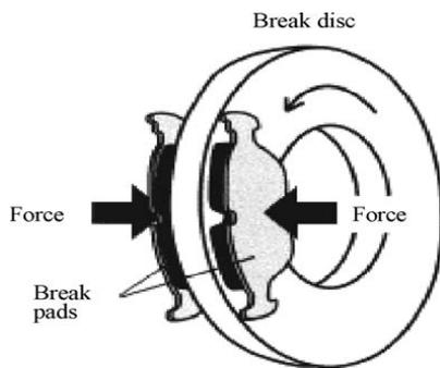
Fig. 2 Schematic view of real size brake system (brake disc and brake pad)
