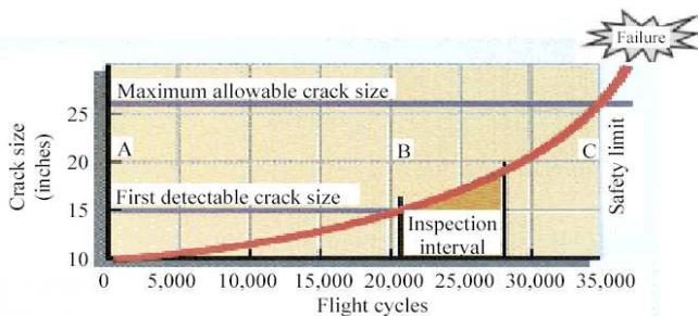
**Fig. 3.** Schematic Fatigue Crack Growth Curve
