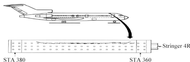
Fig. 2. Example of In-service Cracking from B727 Aircraft
