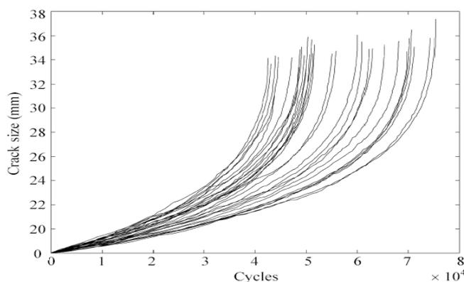
Fig. 1. Constant Amplitude Loading Fatigue Test Data Curves
