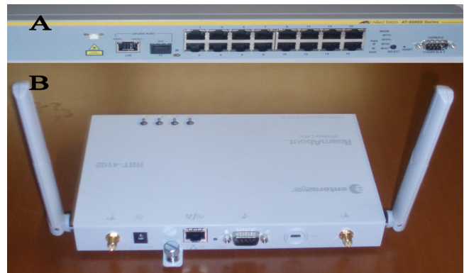
Fig. 1- Switch (A) [14] and access point (B) [13]
