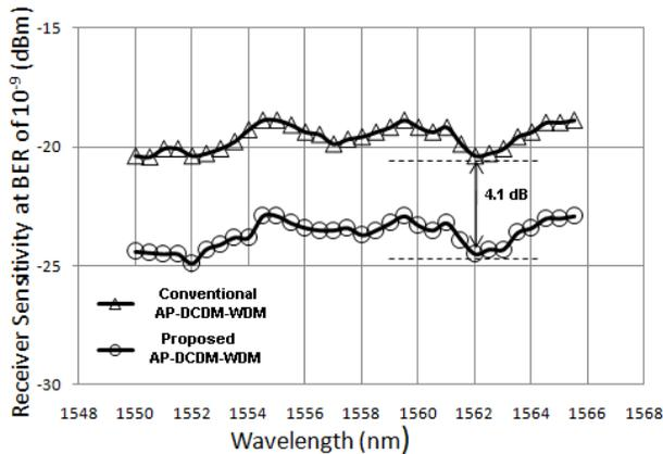
Fig.4 Pre-amplified receiver sensitivity versus signal wavelength for 32 channels
