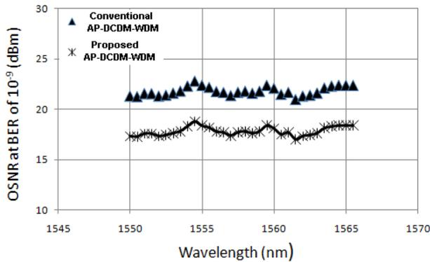
Fig.5. OSNR versus signal wavelength for 32 channels
