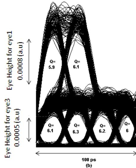
Fig.3 Received eye diagram for channel 16 in 32-channel AP-DCDM-WDM system using optimized DD-MZM
