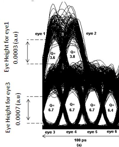
Fig.2 Received eye diagram for channel 16 in 32-channel AP-DCDM-WDM system
