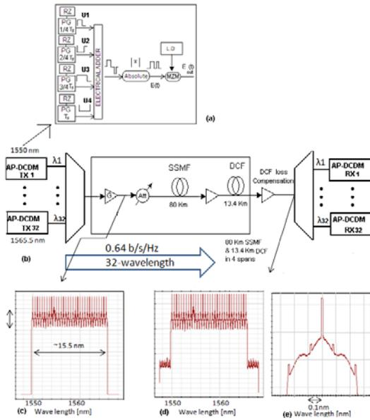
Fig.1. (a) 4 x 10 Gbit/s AP-DCDM transmission system (b) Simulation Setup of 1.28 Tbit/s (32 x 4 x 10 Gbit/s) AP-DCDM-WDM transmissions (c) Optical spectrum before transmission (d) Optical spectrum after transmission (e) single channel AP-DCDM spectrum
