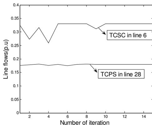
Fig. 12 Modified IEEE 30 bus system with specified line flows in case 2
