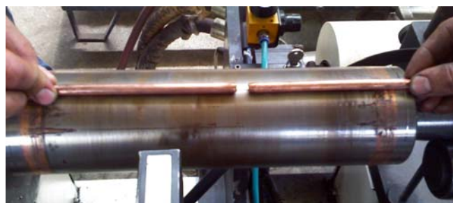
Fig. 3. Photographs of broken rotor bar parts and rotor.
