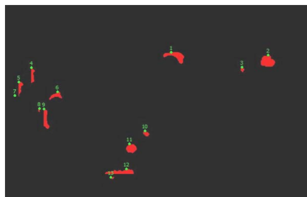
Fig13. Resultant Image of Under etching after Particle Analysis
