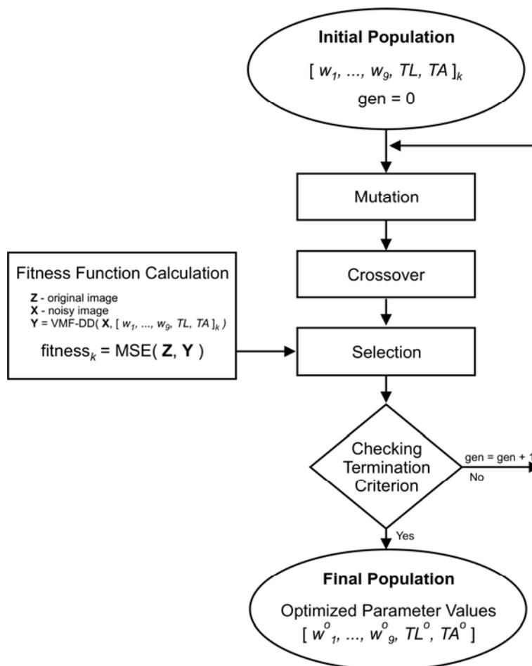
Fig. 2. GA optimization of the VMF-DD parameters
