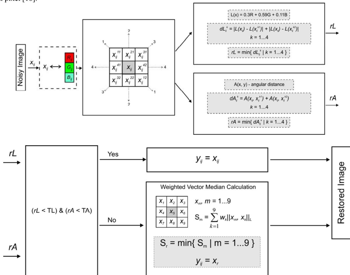
Fig. 1. The scheme of vector median filter with directional detector
