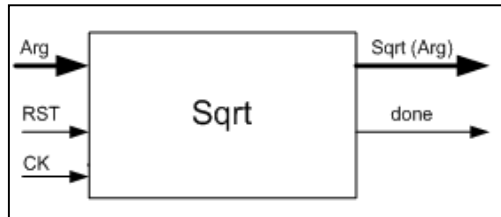
Fig. 6. Top level diagram of the square root operator
