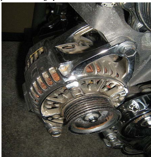
Fig 2: Automotive alternator fixed at the lateral side of an engine.
