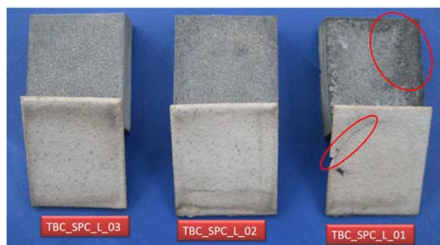
Fig. 1. Specimens after separation of coating layers from substrate in thermal shock test
