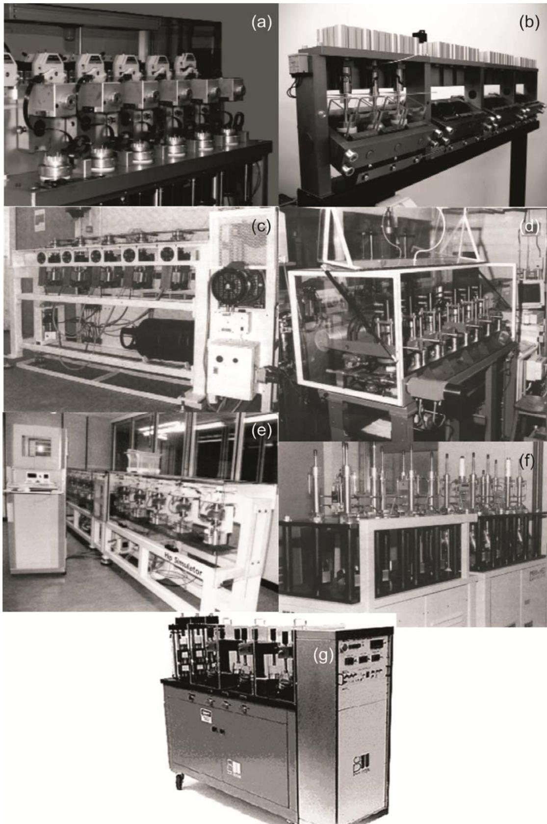
Fig 2: Hip Joint simulators (a) AMTI, (b) HUT-4, (c) Mark II, (d) Leeds PA II, (e) ProSim Limited, (f) MATCO and (g) Shore Western [3]
