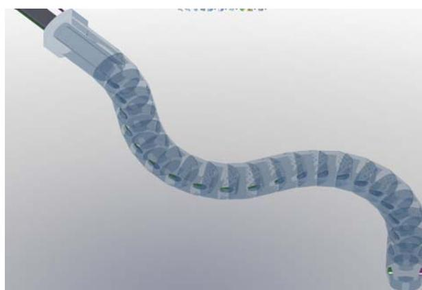
Fig. 7. The poly articulated robotic arm assembly designed with Solid Work 2010 software
