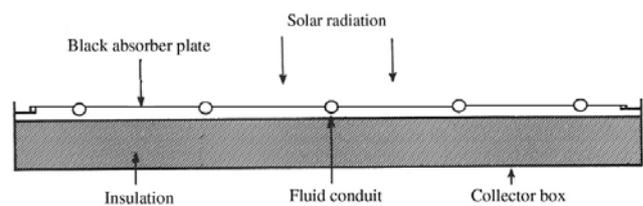
Fig. 1 Cross-sectional view of an unglazed solar flat-plate collector
