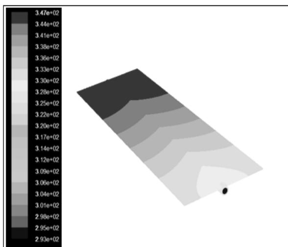
Fig. 10. Temperature plots for unglazed collector without fin for a heat flux of  $800\text{W/m}^2$  and mass flow of  $0.0179\text{kg/min}$
