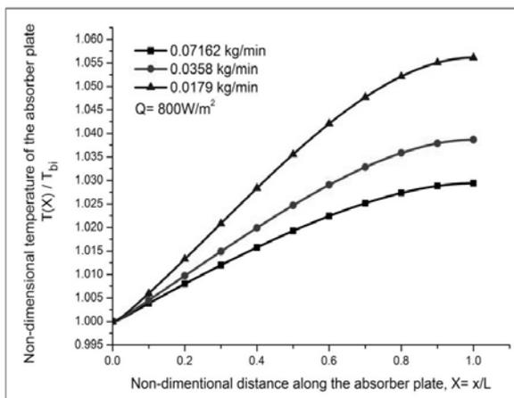
Fig. 7. Temperature plots for three different mass flow rates for the absorber plate without fins in the absorber tube
