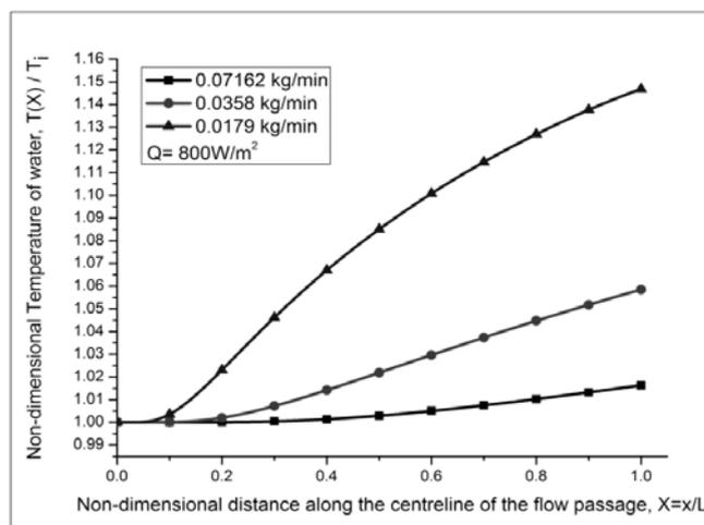
Fig. 6. Temperature plots for three different mass flow rates for the absorber plate without fins in the absorber tube
