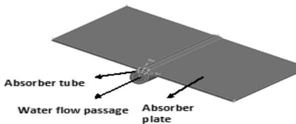
Fig. 2. Geometry of the unglazed collector and absorber Tube without fin (Base model)
