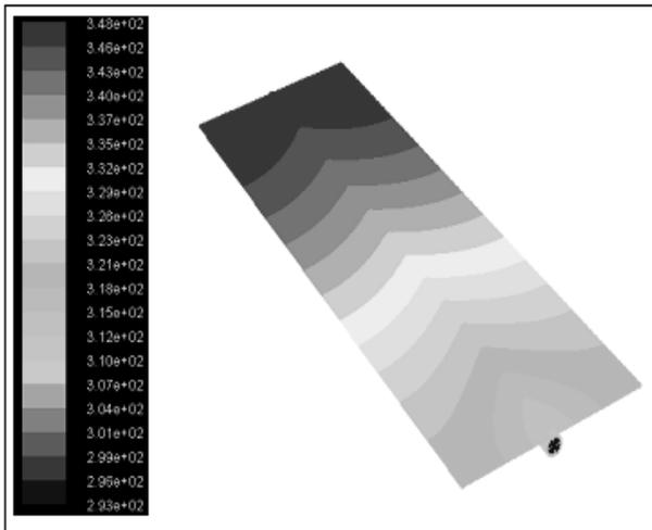
Fig. 12. Temperature plots for unglazed collector with serrated fin for a heat flux of  $800\text{W/m}^2$  and mass flow of  $0.0179\text{kg/min}$
