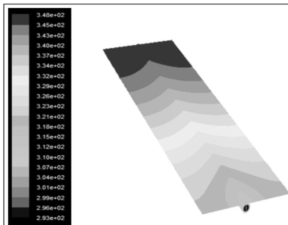
Fig. 11. Temperature plots for unglazed collector with diametrically placed planar fin for a heat flux of  $800\text{W/m}^2$  and mass flow of  $0.0179\text{kg/min}$
