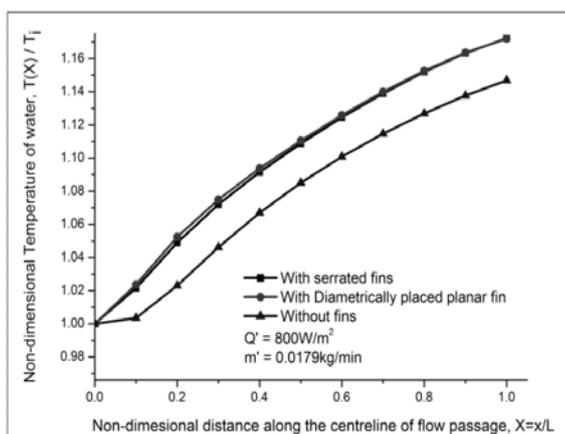
Fig. 8. Comparison of the temperature plots along the centerline of the water flow passage in the absorber tube with and without fins
