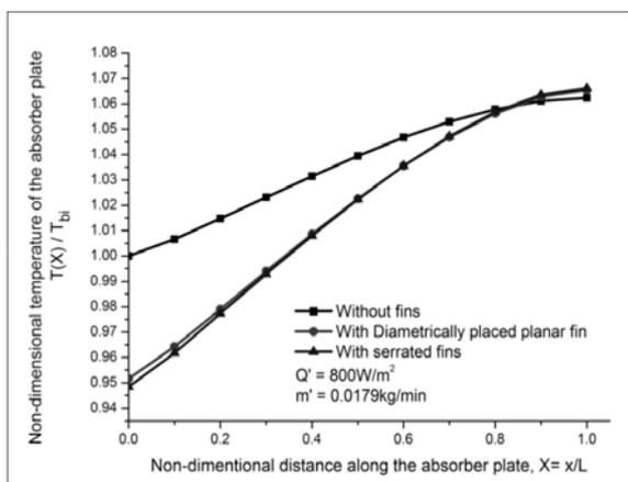
Fig. 9. Comparison of the temperature plots along the length of the absorber plate having absorber tube with and without fins
