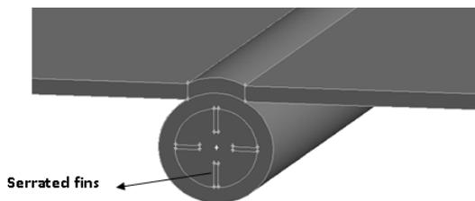
Fig. 4. Geometry of the unglazed collector and absorber Tube with serrated fins.
