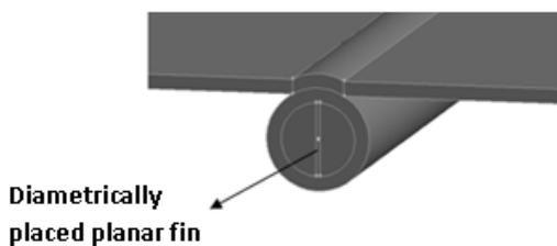
Fig. 3. Geometry of the unglazed collector with Diametrically placed planar fin
