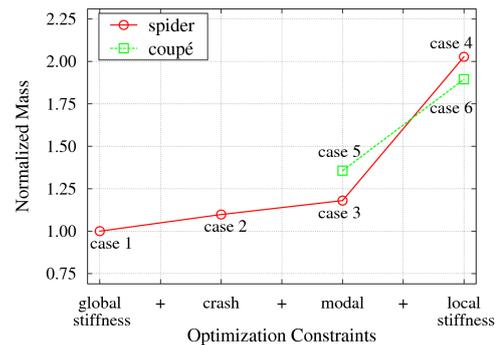
Fig. 2. Trend of the chassis mass as constraints are added to the topology optimization process; the mass is normalized over the mass of case 1. The masses for cases 5 and 6 include the mass of the roof.
