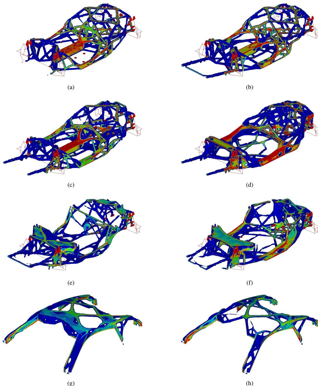
Fig. 3. Topology optimization results: figures (a) to (f) refer to cases 1 to 6 respectively; (g) and (h) are the roofs obtained for cases 5 and 6. The different colours stand for different material relative densities with blue being 10% and red 100%. Elements with relative density lower than 10% are not shown.
