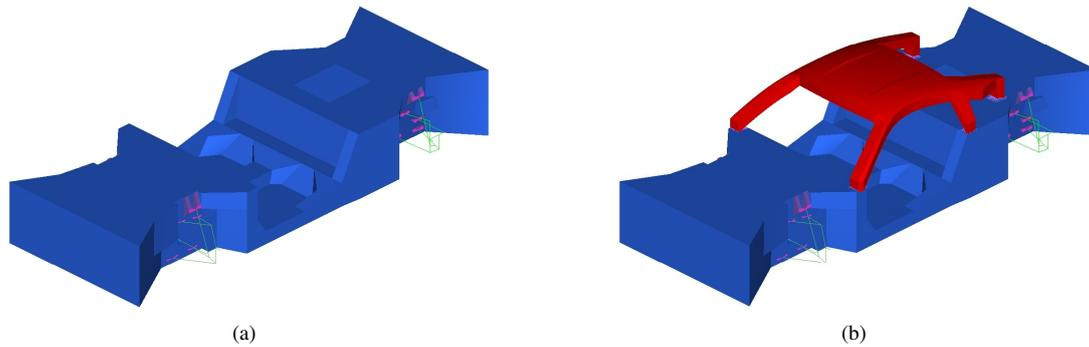
Fig. 1. Topology optimization domains: (a) spider vehicle chassis, (b) coupé vehicle chassis.
