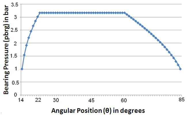
Fig. 4. Pressure profile inside the bearing w.r.t. Angular position.
