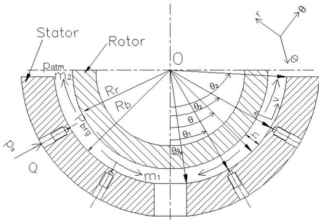
Fig 2: Sectional View of Hemispherical Air Bearing
