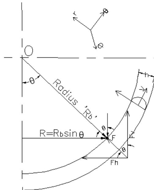
Fig 3: Geometry of Spherical Bearing
