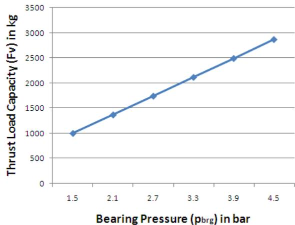
Fig 5. Bearing Pressure Vs Thrust Load Capacity of the spherical bearing.
