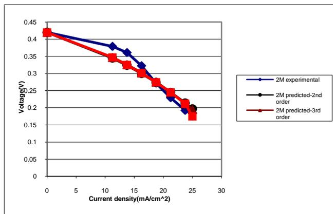
Fig 9: Experimental vs. Predicted polarization curve for 2M methanol solution
