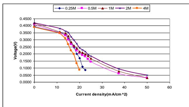
Fig 1: Polarization curve showing the effect of methanol concentration [6].
