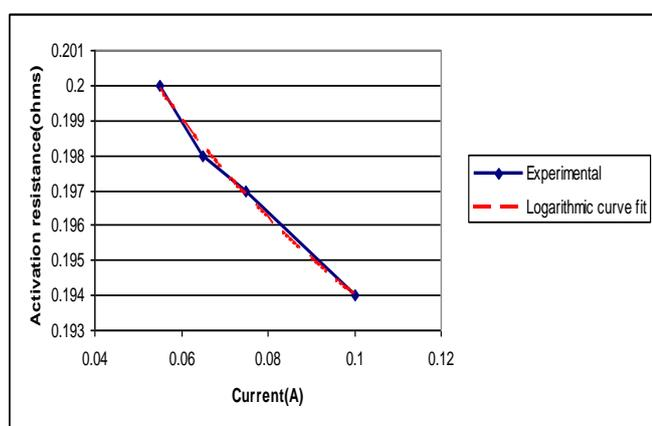
Fig 6: Activation losses vs. current for 4M methanol solution
