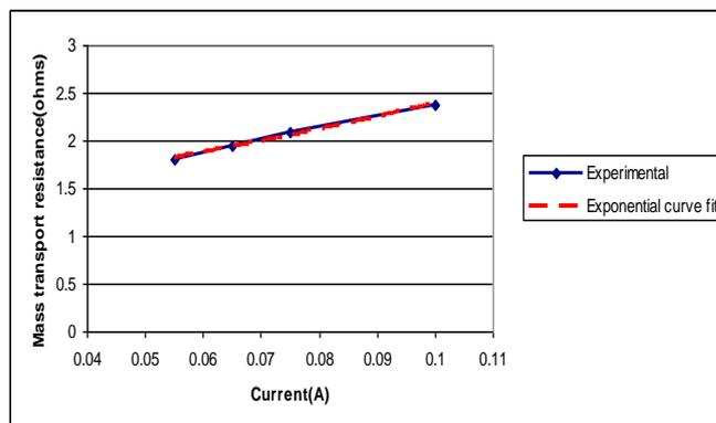
Fig 7: Mass transport losses vs. current for 4M methanol solution
