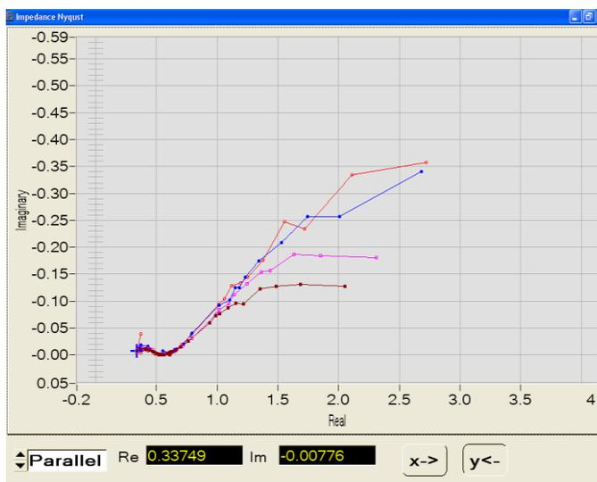
Fig 4: Nyquist plot generated for 0.25M methanol concentration [6].
