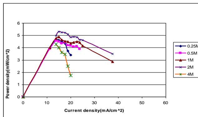
Fig: 2 Power density curves at different methanol concentrations [6].
