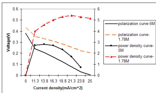
Fig 10: Simulated polarization and power density curve for 5M & 1.78M methanol solution
