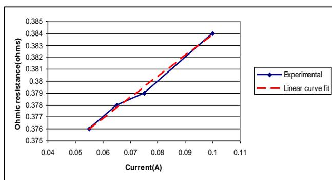
Fig 5: Ohmic losses vs. current for 4M methanol solution
