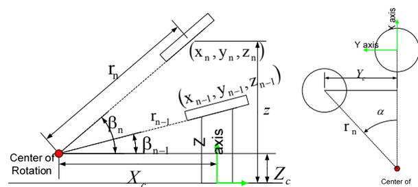
Fig 3. Side view of experimental setup (left); and the displacement of center of rotation during valgus and varus motion on XY plane (right)
