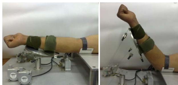
Fig.1. Stewart platform based elbow joint measurement device and arm fixation apparatus
