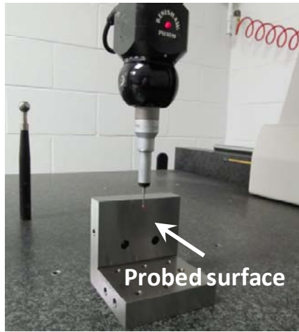
Fig. 6. Setup for the single configuration repeatability test.
