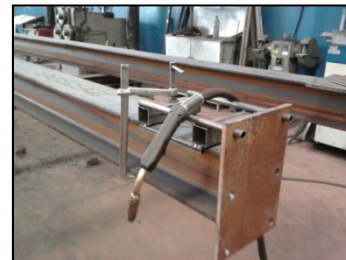
Fig.11. Mistake proofing mechanism for frames assembly
