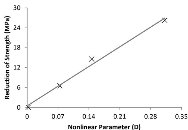
Fig. 4. Correlation between reduction of compressive strength and nonlinearity parameter
