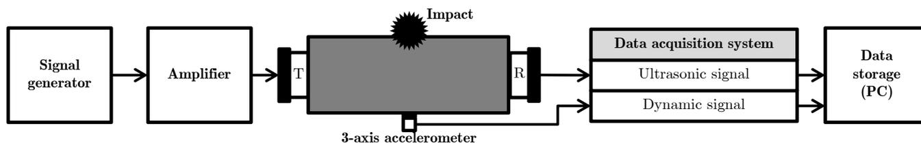
Fig. 1. Schematic diagram of nonlinear ultrasonic modulation technique
