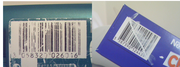
Fig. 1. Low quality and damaged image barcodes
