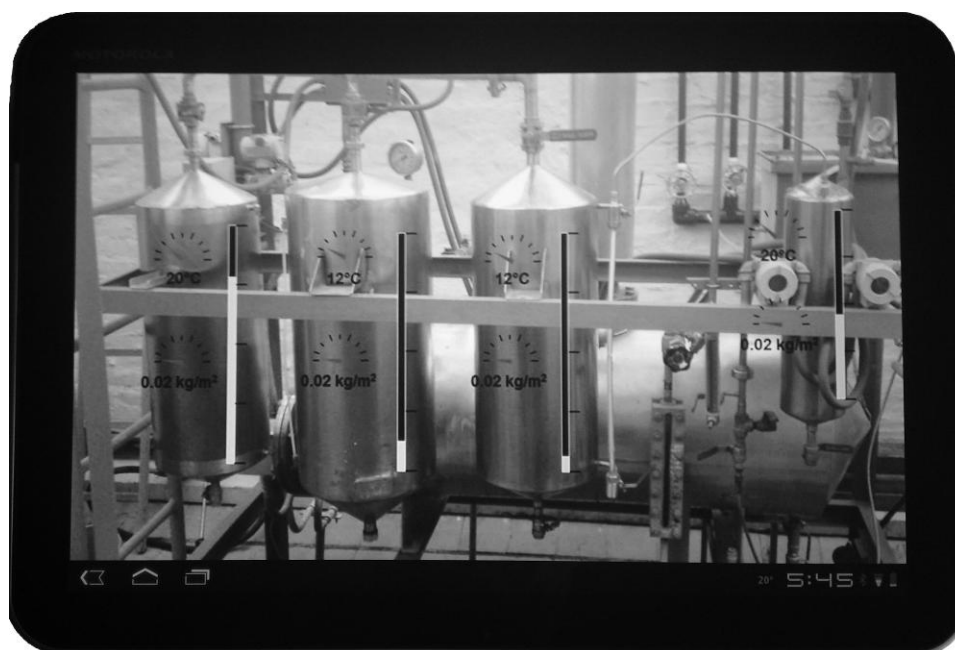
Fig. 4. Conceptual prototype applied on a discontinuous distillation plant (level, temperature and press gauges as additional virtual objects).
