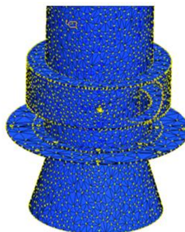
Fig 6: Meshing/Discretization of the developed Recuperative Heat Exchanger
