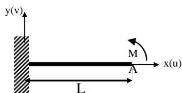
Fig 5 Cantilever beam with end moment, and beam properties
