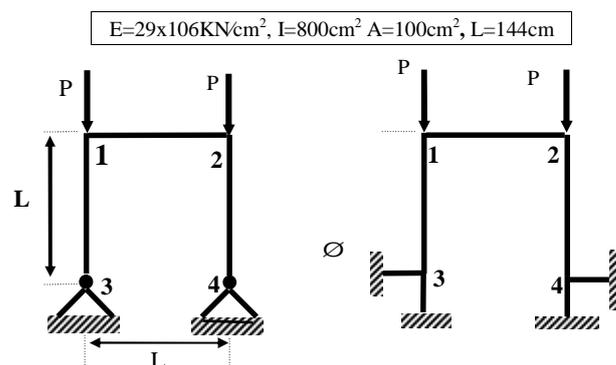
Fig 6 Plane frame buckling A
