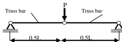
Fig 1 Geometrically Unstable Structure
