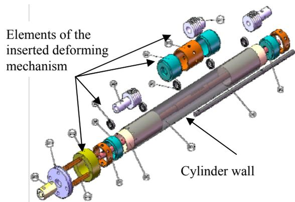
Fig.1. Exploded view of the circular cylinder maquette
