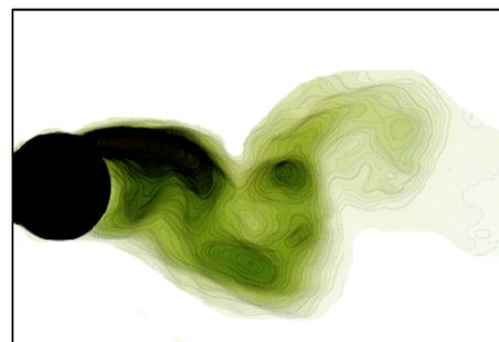
Fig.2. Flow around a circular cylinder / natural evolution,  $Re=2700$ .
