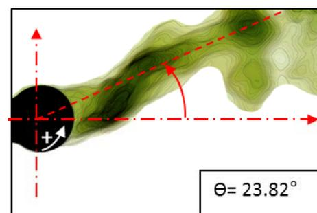
Fig.3. Flow around a rotating cylinder,  $\alpha=2.26$  and  $Re=2700$ .
