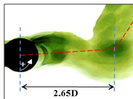
Fig.4. Flow around a rotating and radially deforming cylinder,  $\alpha=2.26$ ,  $f_s=3.34$  and  $Re=2700$ .
