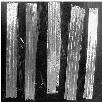
Fig. 5. Al- Basalt laminates for hot pressing.
