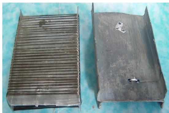
Fig. 3. A fixture before and after winding.
