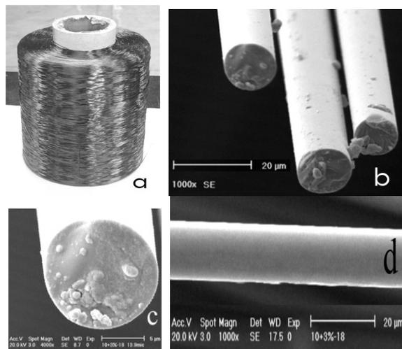
Fig.1. a) A reel and b,c,d) SEM micrographs of Basalt fibers
