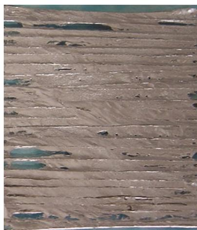
Fig. 4. A laminate after separating from its fixture.
