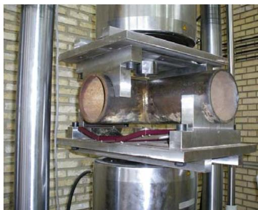
Fig. 2 The fixture and the specimen on place
