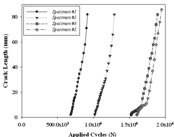
Fig.5 Crack length versus fatigue life of tubular X-joints;  $R=0.1$ ,  $\sigma=265$  MPa,  $f=5$  Hz; ( simple joints: specimens 1 and2 and shot peened joints: specimens 6, 5)
