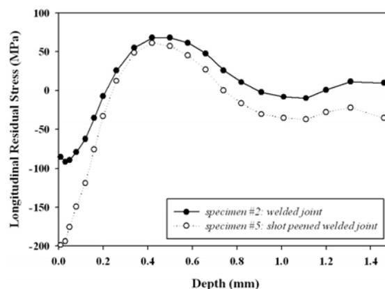
Fig. 3 Distribution of residual stress on Specimen #2 (welded joint), before and after the fatigue test
