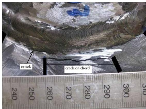
Fig. 6 Cracked joint
