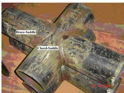
Fig. 1: Welded X-joint
