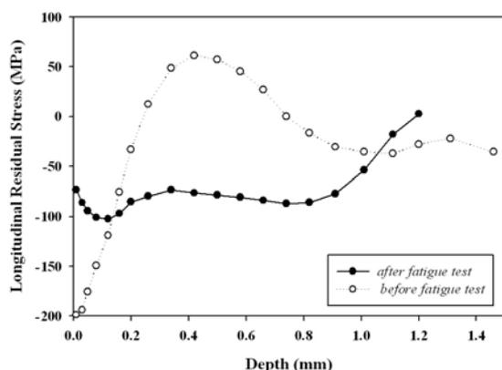
Fig. 4 Distribution of residual stress on Specimen #5 (shot peened welded joint), before and after the fatigue test
