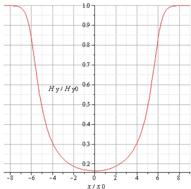
Fig. 3. Normal component of the field strength for the case  $b_0 = 12 \delta$ .
