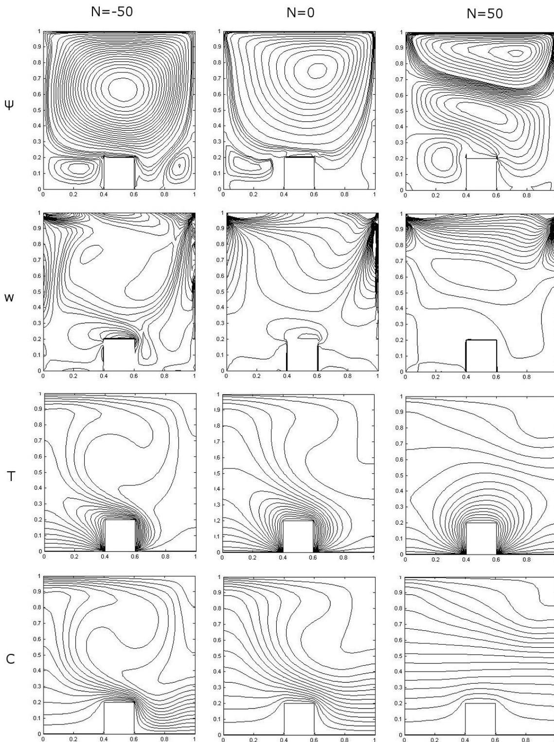
Fig. 2. The effect of the buoyancy forces for  $Ri = 0.1$ ,  $Re = 100$
