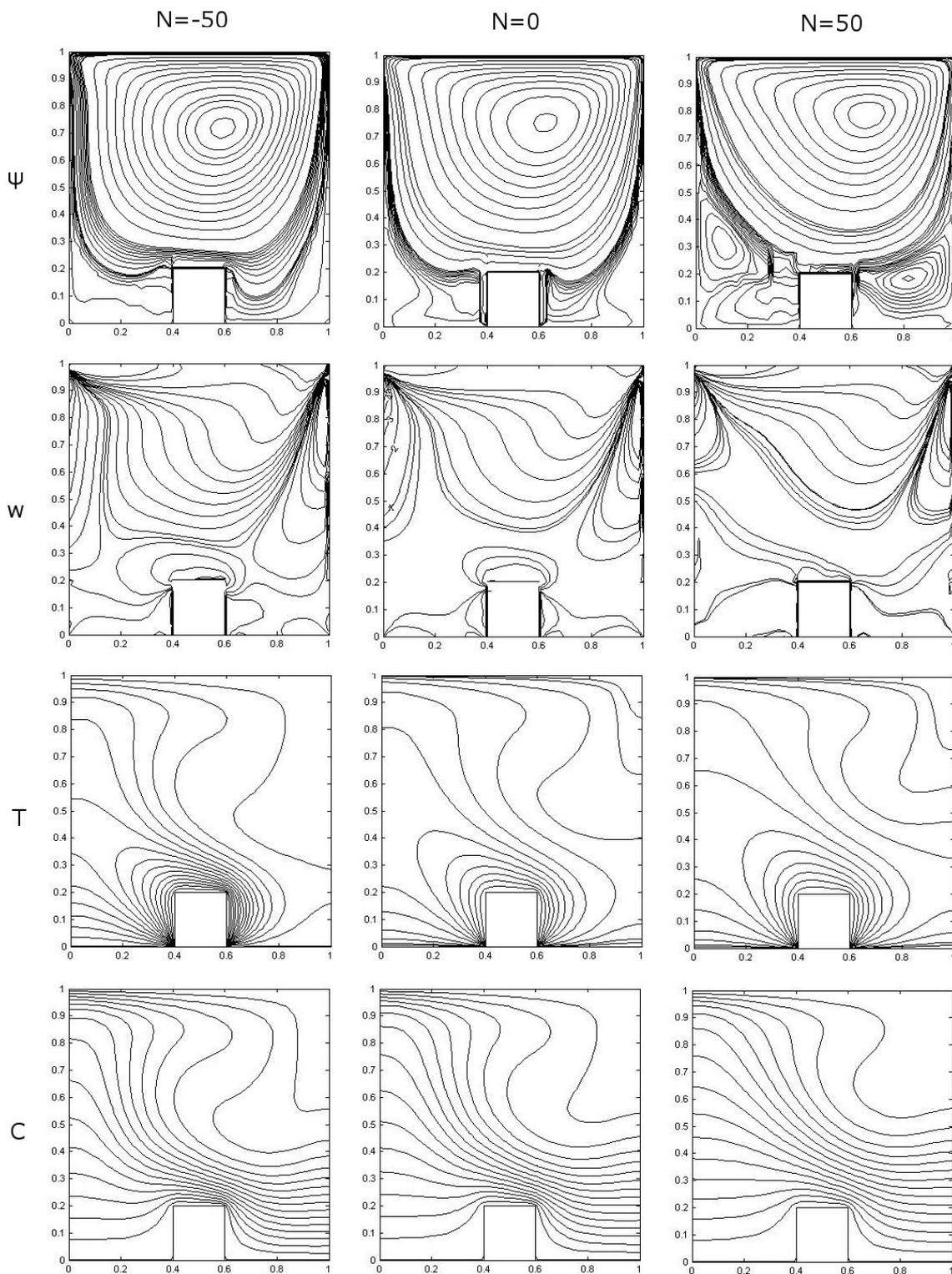
Fig. 1. The effect of the buoyancy forces for  $Ri = 0.01$ ,  $Re = 100$
