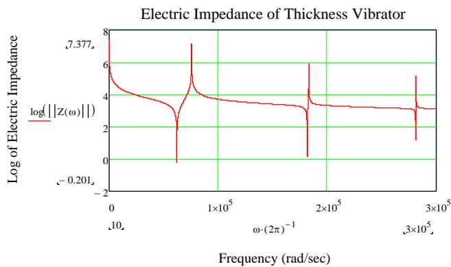
Fig.3. Graph of electric impedance (in logarithmic scale) versus frequency.
