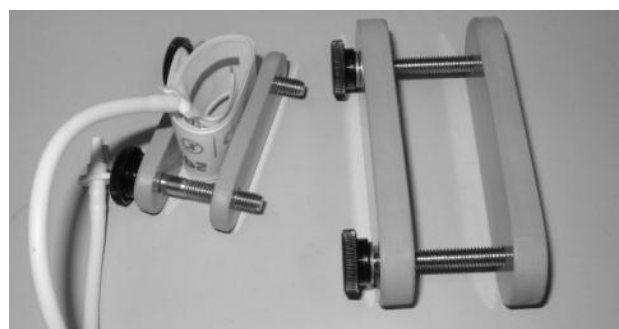
Fig. 4. Tongue 'clamps' for maintaining natural tongue shape during occlusion.
