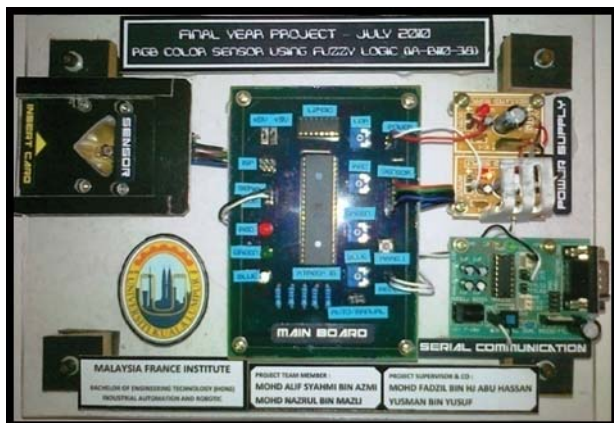
Fig. 18. The RGB colour classification using Fuzzy Logic kit.
