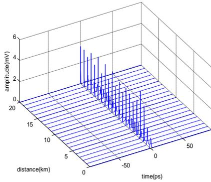
Fig 6: Pulse evolution of nonlinear effect on ultrafast pulse at a distance of 20 km
