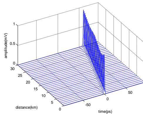
Fig 11: Pulse evolution combined effect of dispersion and nonlinear effect at a distance of 30 km
