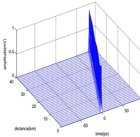
Fig 12: Pulse evolution of the combined effect of dispersion and nonlinear effect at a distance of 40 km
