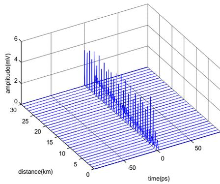
Fig 7: Pulse evolution of nonlinear effect on ultrafast pulse at a distance of 30 km
