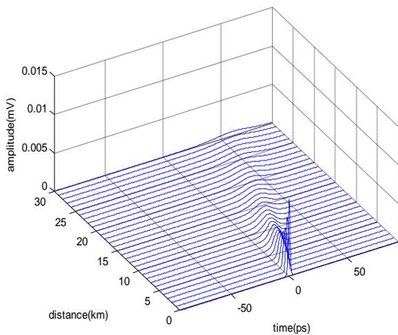
Fig 3: Pulse evolution of dispersion effect on ultrafast pulse at a distance of 30 km
