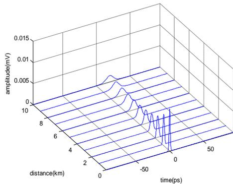
Fig 1: Pulse evolution of dispersion effect on ultrafast pulse at a distance of 10 km
