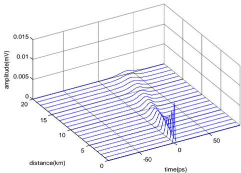
Fig 2: Pulse evolution of dispersion effect on ultrafast pulse at a distance of 20 km
