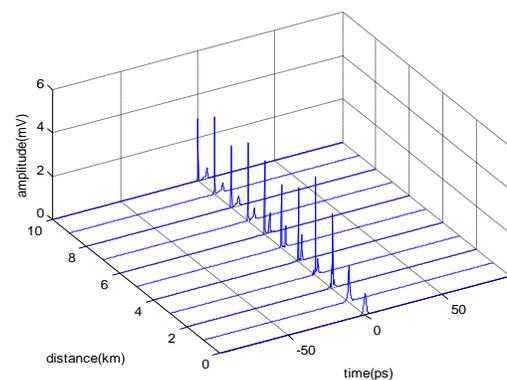
Fig 5: Pulse evolution of nonlinear effect on ultrafast pulse at a distance of 10 kilometers
