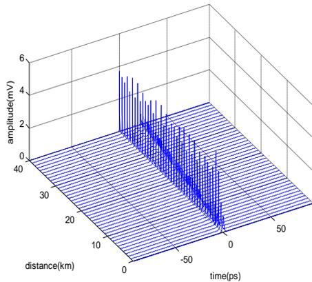
Fig 8: Pulse evolution of nonlinear effect on ultrafast pulse at a distance of 40 km
