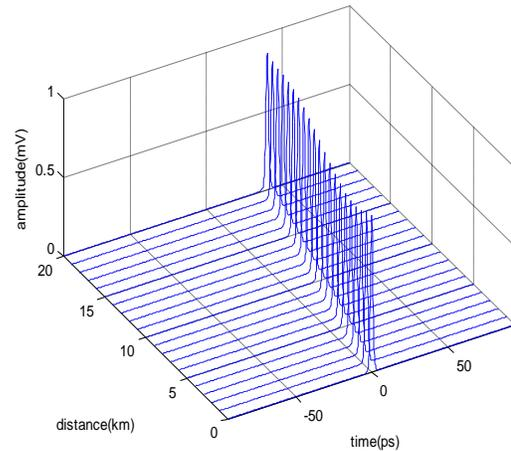
Fig 10: Pulse evolution combined effect of dispersion and nonlinear effect at distance of 20 km
