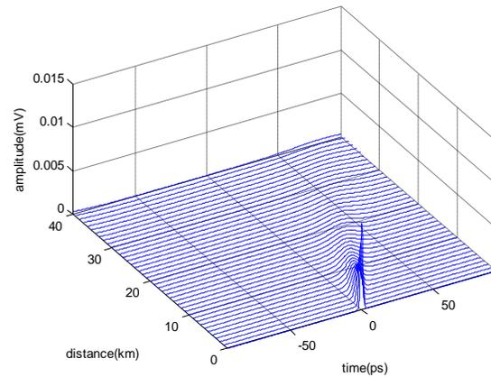
Fig 4: Pulse evolution of dispersion effect on ultrafast pulse at a distance of 40 km
