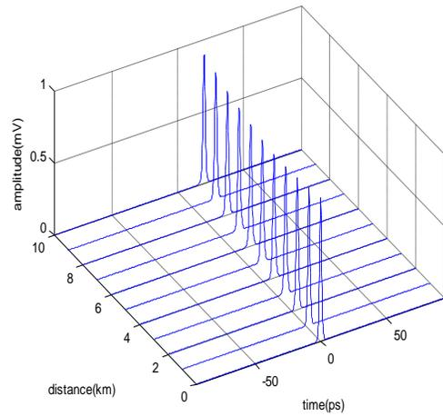
Fig 9: Pulse evolution combined effect of dispersion and nonlinear effect at a distance of 10 km
