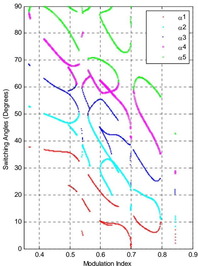
Fig 7. Switching angles for an 11-level CMLI for Case III.
