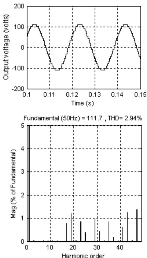
Fig 12. Simulated output line voltage (top) and its harmonic spectrum for 11-level CMLI at  $m = 0.8445$  for Case III.
