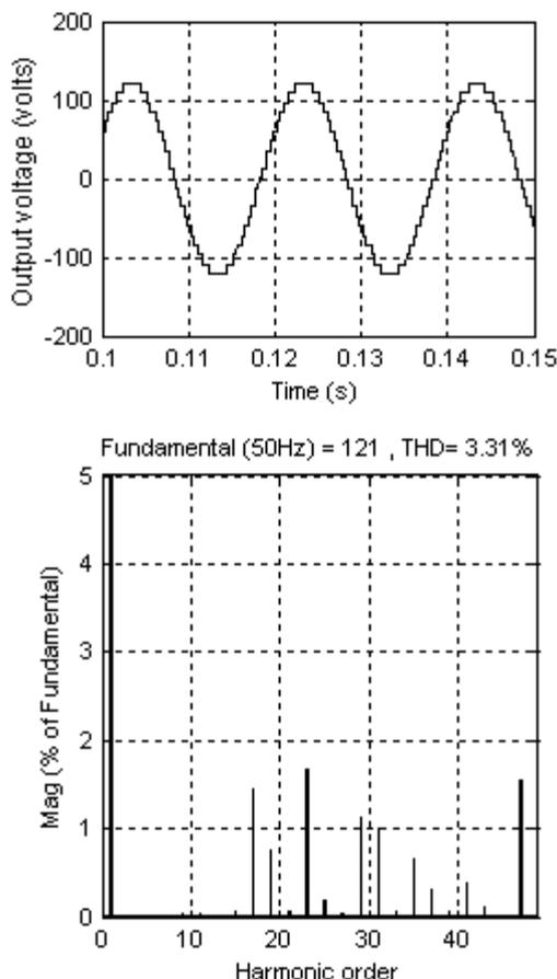
Fig 11. Simulated output line voltage (top) and its harmonic spectrum for an 11-level CMLI at  $m = 0.9145$  for Case II.
