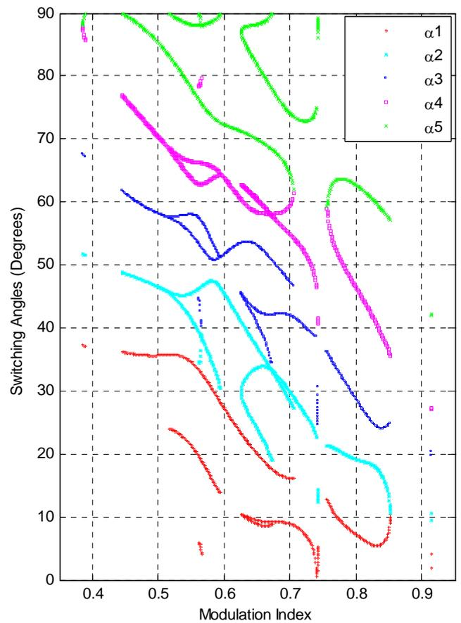
Fig 5. Switching angles for an 11-level CMLI for Case II.
