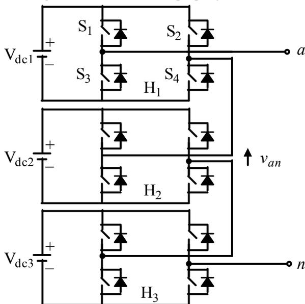
Fig 1. Configuration of seven-level CMLI with unequal dc sources.
