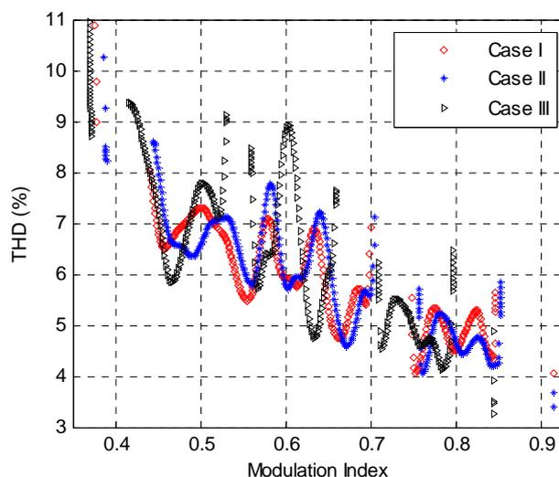
Fig 10. THD<sub>49</sub> for first solution set under three cases.
