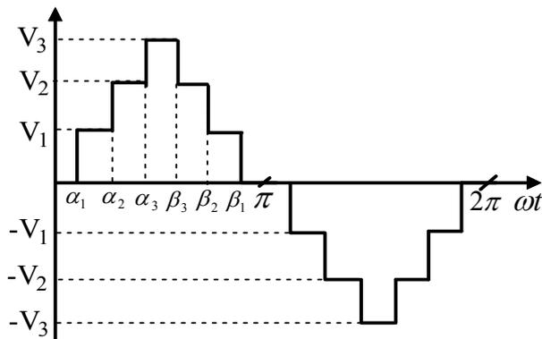
Fig 2. Typical output voltage waveform for a 7-level CMLI.
