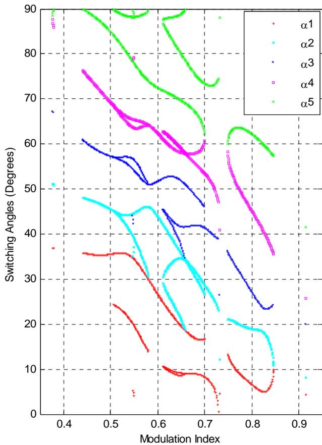
Fig 3. Switching angles for an 11-level CMLI for Case I.
