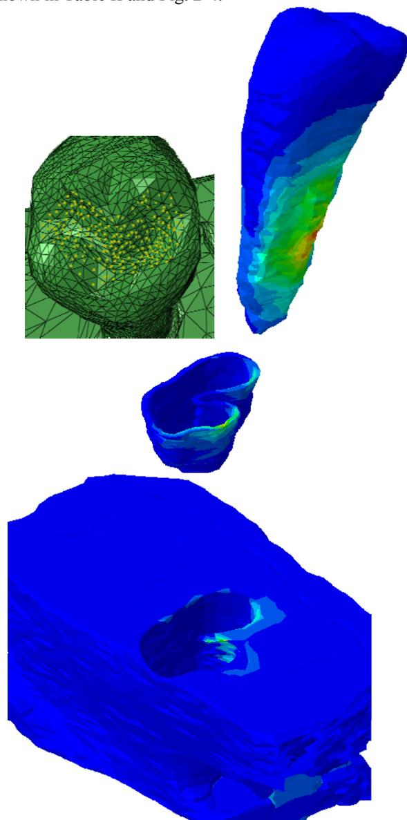
Fig. 1. presents the strain distribution within the all 3 model's components (tooth, PDL and bone) and the occlusal applied load
