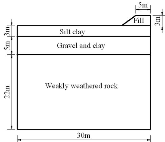
Fig.1 Profile of embankment computational model
