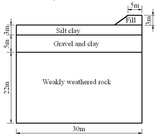
Fig.1 Profile of embankment computational model
