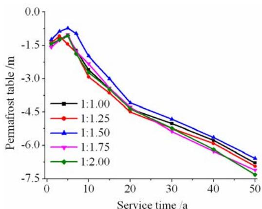
Fig.4 The permafrost table changes with time under different slope gradient
