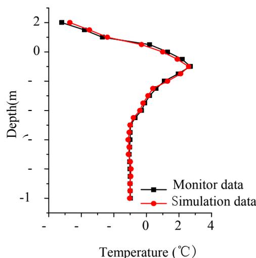
Fig.2 Measured and calculated temperature values at the maximum thawed depth of embankment centre
