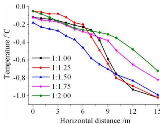
Fig.6 The horizontal distribution of ground temperature at the depth of 3 meters on September 15<sup>th</sup> of the fiftieth year
